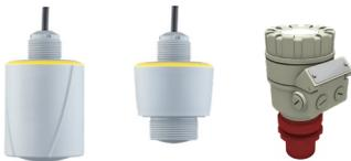
The radar velocity sensors are operating at the free 24 GHz band frequency and make use of the Doppler effect to gain information about the speed of the moving surface. The sensor does this by beaming a microwave signal to the flow surface at a defined angle and analyzing the signal reflection from particles and disturbances moving with the flow. The frequency of this returning signal has been shifted by an amount directly proportional to the spot velocity.
