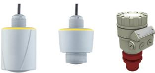
The ultrasonic level sensor operates by energizing a piezoelectric transducer with an electronic pulse. This pulse creates a pressure wave that travels to the flow surface and is partially reflected back to the transducer. The signal time of flight to the flow surface and back is recorded. The actual distance is calculated knowing the speed of sound at the site, which is corrected by an embedded temperature sensor.
