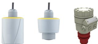
The ultrasonic level sensor operates by energizing a piezoelectric transducer with an electronic pulse. This pulse creates a pressure wave that travels to the flow surface and is partially reflected back to the transducer. The signal time of flight to the flow surface and back is recorded. The actual distance is calculated knowing the speed of sound at the site, which is corrected by an embedded temperature sensor.
